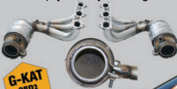
KIT2 (-7.5Kg) Special quiet version for racetracks with noise restrictions Part-No.: CARP97GT3KIT2
